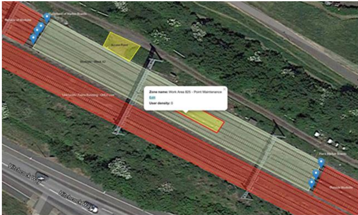
Figure 1 – Geofence safe and unsafe zone example
